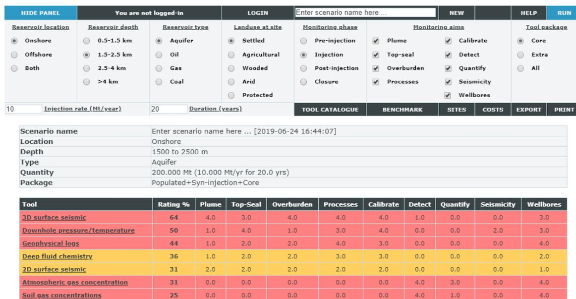
Figure 2-10. Snapshot of recommendations for IEAGHG monitoring tool package to be implemented in an aquifer during the CO<sub>2</sub> injection phase for the selected monitoring objectives. The monitoring tools in Red are ones identified to have been assigned the highest scores across the selected aims and are strongly recommended techniques (Score 4).
