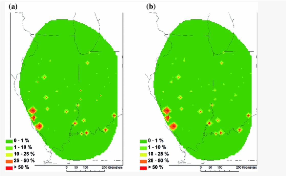
**Figure 2-6. CO<sub>2</sub> saturation simulated in the Arkosic Unit of the Mount Simon based on the refined stratigraphy model after a) 50 years, b) 100 years [Bandilla et al., 2012].**
