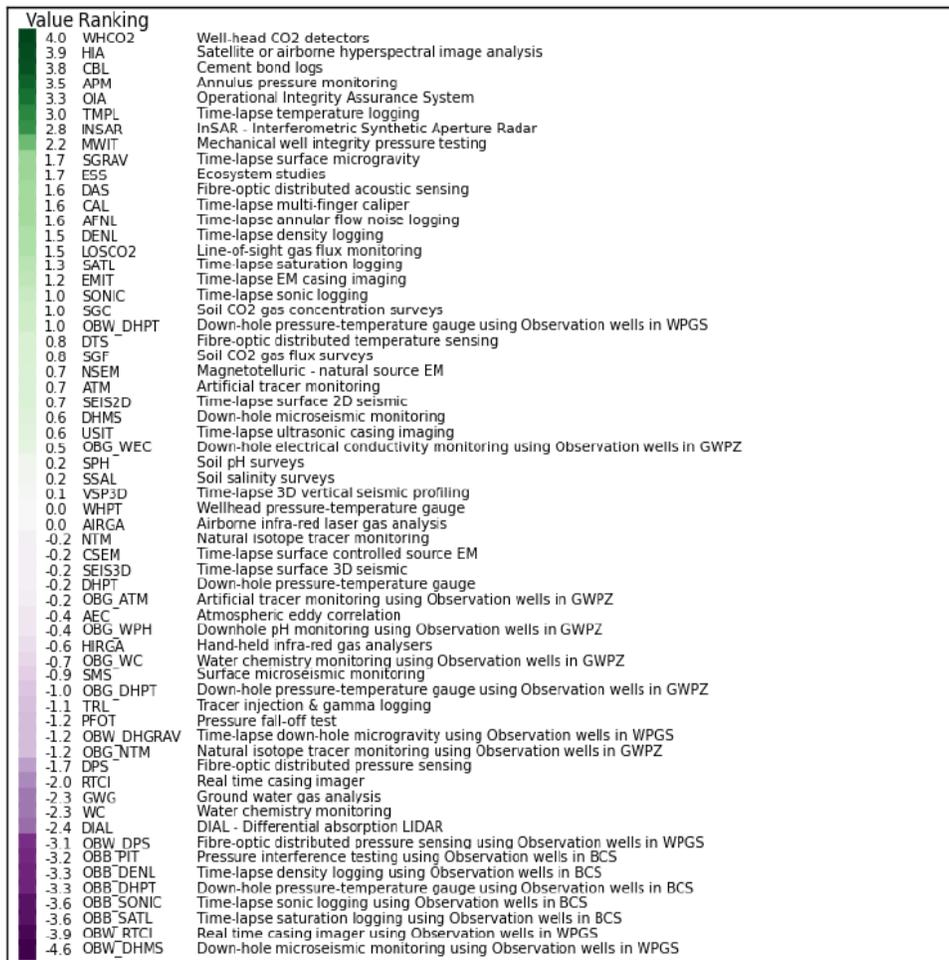
**Figure 2-8. Cost-benefit ranking of monitoring technologies evaluated in the Shell QUEST CCS project [Shell, 2010]. Colours denote the difference between the benefit and cost rankings as an indicator of value.**
