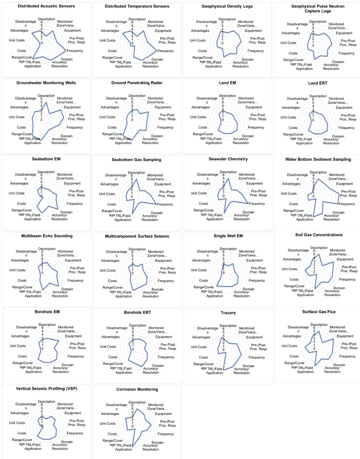
Figure 2-5A continued. Radar plots for surface/near-surface CO<sub>2</sub> storage monitoring technology cost-benefit metrics.
