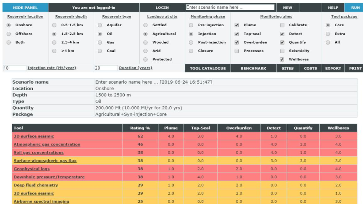
Figure 2-11. Snapshot of recommendations for IEAGHG monitoring tool package to be implemented in an oil field during the CO<sub>2</sub> injection phase for the selected monitoring aims. The monitoring tools in Red are ones identified to have been assigned the highest scores across the selected aims and are strongly recommended techniques (Score 4).
