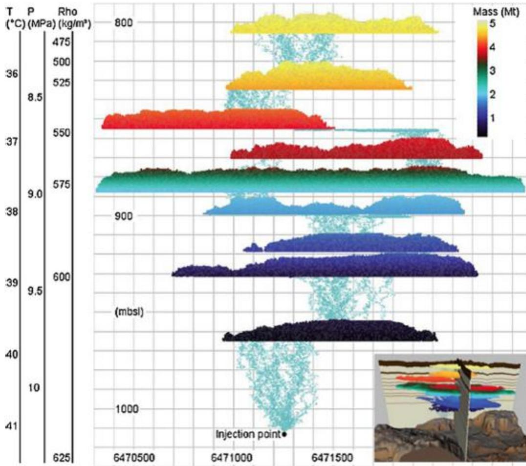
**Figure 2-7. Simulation CO<sub>2</sub> migration at the Sleipner injection site using an alternative flow physics model [Cavanagh and Haszeldine, 2014].**
