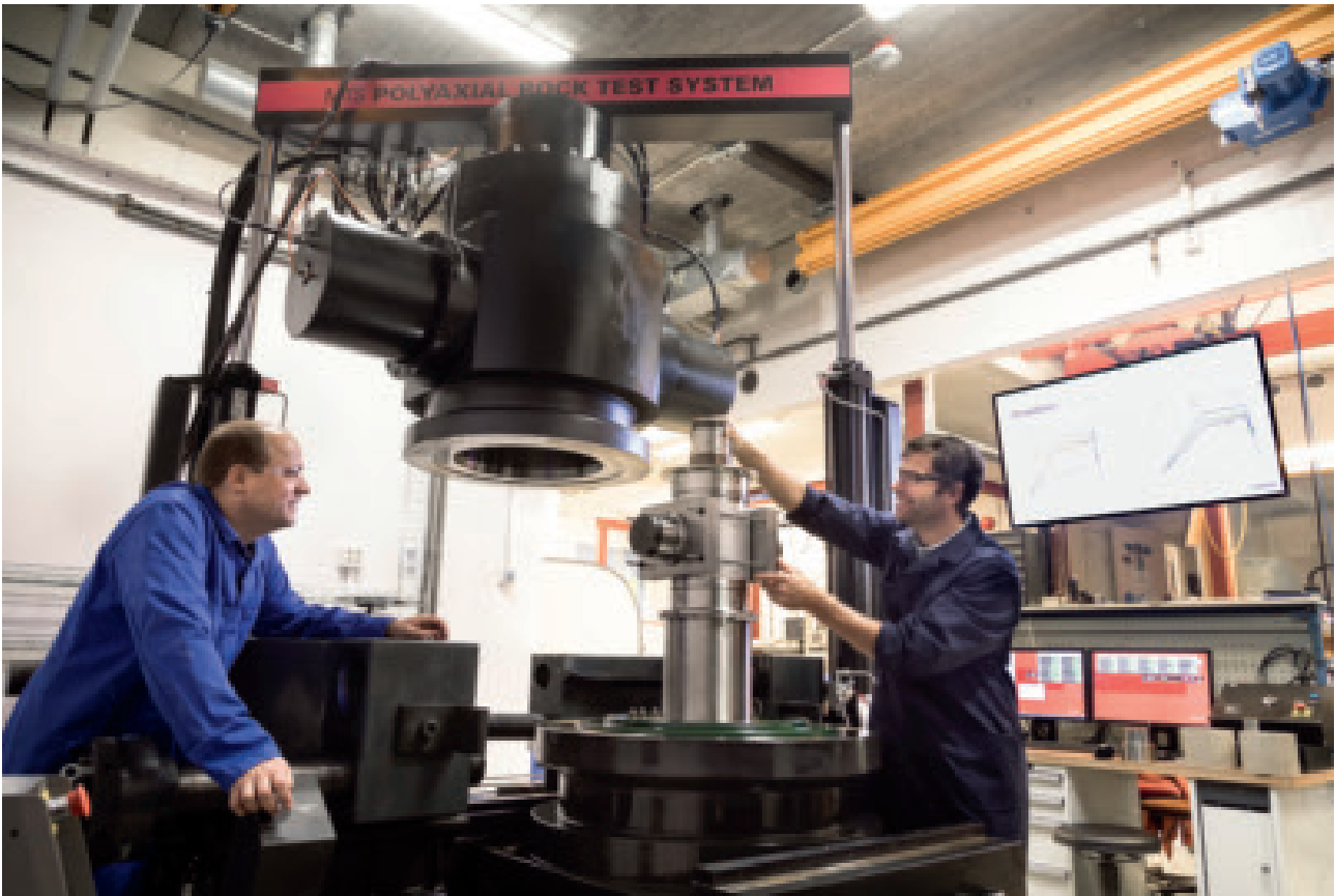
Small scale wells are tested under realistic pressure and temperature conditions with specialized equipment. Photo: SINTEF.
